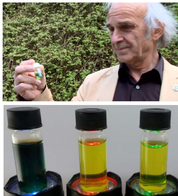
Figure 4. In direct sunlight and blue LED light, the yellow PBB solution turns blue (see reactions in the yellow box in Figure 5); however, there is no blue coloration when irradiated with red or green light
