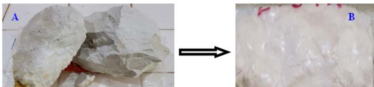
Figure 1. Clay transformation: Raw clay (A) and elaborated geopolymer (B)
