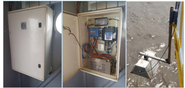
Figure 4. Electronic control box of a tide station and external radar sensor under protection
