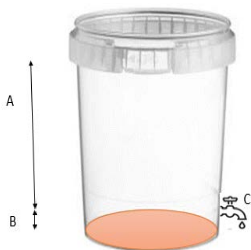
Figure 2. Iron removal device (A: Precipitation unit, B: Iron hydroxide deposition, C: Treated water recovery valve)
