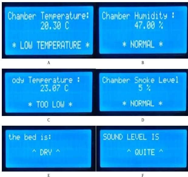
Figure 8. LCD interface with (letter A): A) chamber temperature B) chamber humidity C) body temperature D) chamber smoke level E) liquid sensor F) sound level
