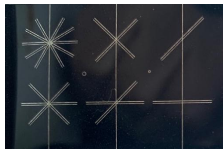
Figure 4.1. Diaphragms of single slit crossing single slit and single slit crossing double slit
