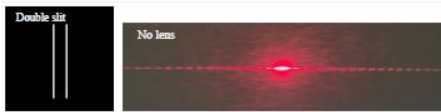
Figure 3.3. Double slit and interference pattern: no lens
