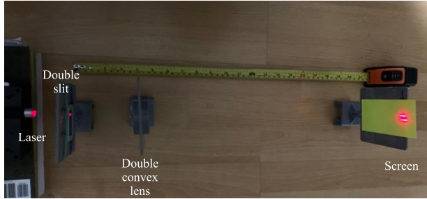
Figure 3.4. Experiment: L = 100 mm
