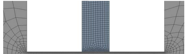
Figure 11. Schematic diagram of the simulated two dimensional model with partial structural meshing.
