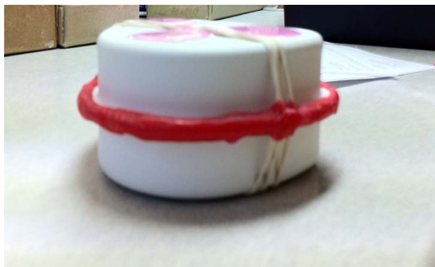
Figure 7. The lab putty mold portions were reassembled and held together with rubber bands
