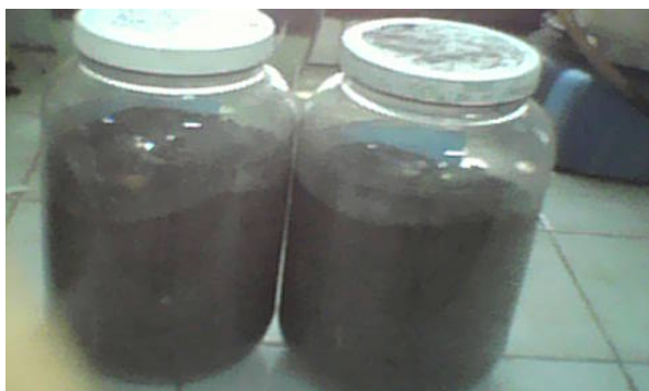
Figure 3. Ashes obtained after burning Landfill C waste
