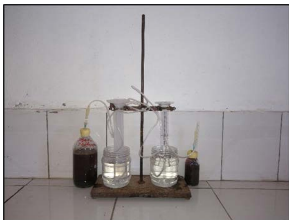
Figure 3. Device for producing biogas and methane volumes
