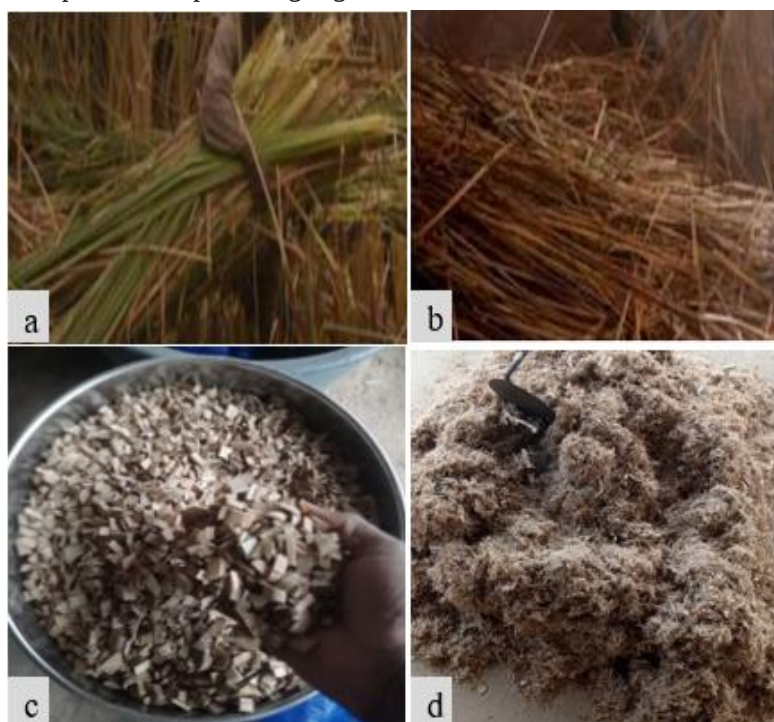
Figure 1. Typha stems (a) harvested, (b) dried, (c) chopped, (d) ground
