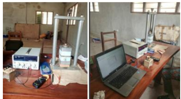
Figure 7. Measurement setup of the asymmetric guarded hot plate method
