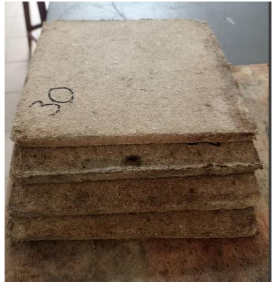
Figure 9. Panels obtained at each compaction pressure: 3 MPa, 10 MPa, 20 MPa, 30 MPa
