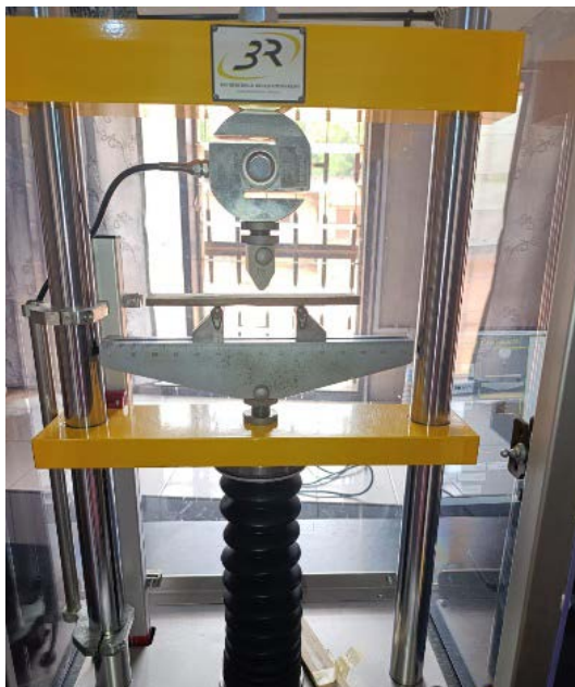
Photo 3. Three-point bending test on bamboo strips
