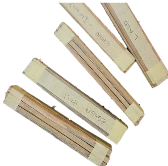
Photo 2. Bamboo strips (20 cm × 3 cm × 1 cm) prepared for testing
