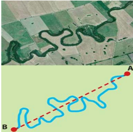
Figure 2. Schematic representation of the sinuosity index calculation for a river reach
