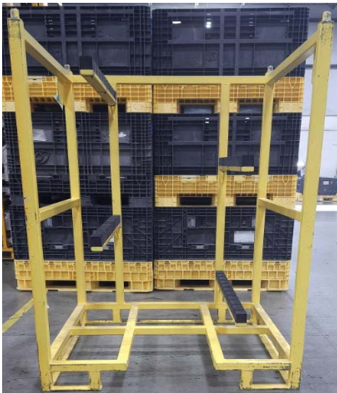
Figure 4. Old rack structure which was common for right and left side door causing surface B to be exposed for right side door
