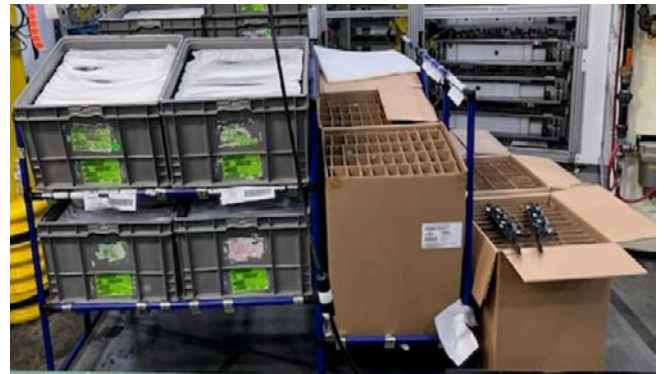
Figure 7. Old rack structure for storing speaker grille and decos which made it difficult to return the empty crates
