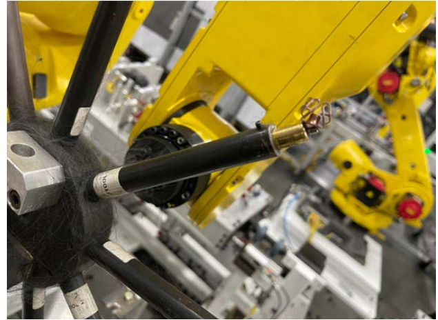
Figure 9. Incorrect orientation of pushnut arising from improper magnetization of surface
