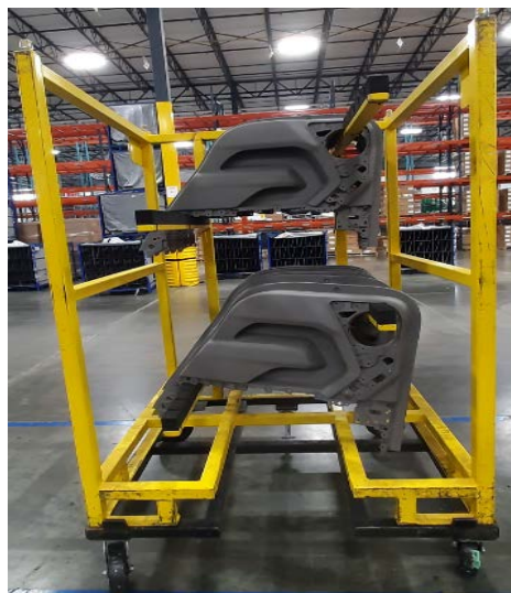
Figure 5. Right hand Rear Door in new rack structure. Door side A is exposed which helps team member to inspect door while removal and reduces extra operation of turning the door over
