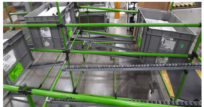
Figure 8. New rack structure used sliding mechanism which made it convenient for team member to return the empty crates
