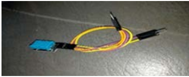
Figure 9. Temperature and humidity sensor
