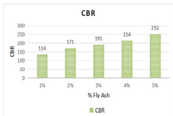
Figure 5. California Bearing Ratio (CBR) of Laterite Improved with 4% Fly Ash and Cement
