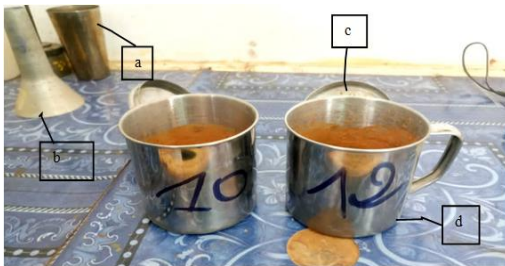
Figure 9. Equipment for testing organic matter content
