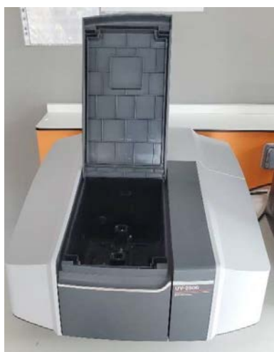
Figure 3. UV-visible spectrophotometer used for adsorption test
