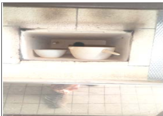
Figure 2. Ceramic crucibles containing calcined soils in the furnace
