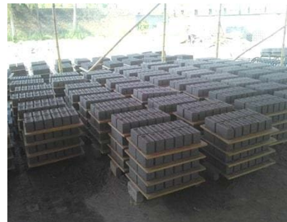
Figure 3. The stacking of Calcium Silicate Bricks
