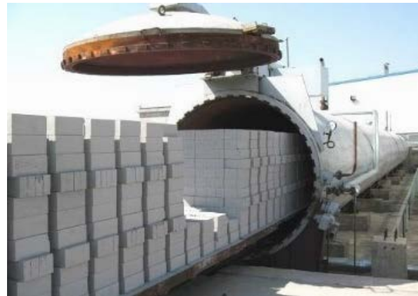
Figure 2. The 20m long steel cylinder act as an Autoclave
