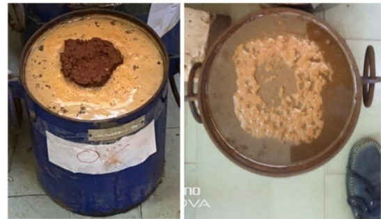
Figure 7. Total immersion of unstabilized CEB
