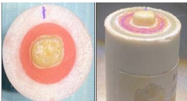
Figure 1. Prepared primary second molar teeth fixed in plastic tubes with auto polymerizing acrylic resin
