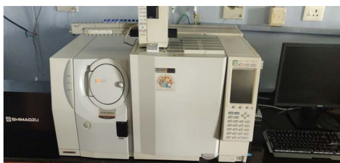
Figure 6. SHIMADZU's GCMS-QP2010 SE with a Capillary Column (0.25 mm \times 30.0 m \times 0.25 \mu m)
