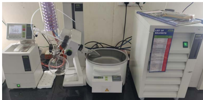
Figure 5. Rotavapor evaporating, to remove the solvent from the flower sample
