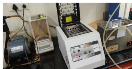
Figure 4. Ultrasonication removes the dirt and makes the samples solvable by breaking the bonded particles
