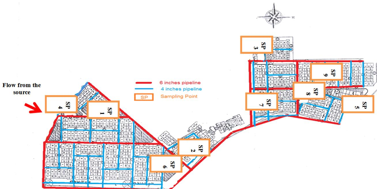
Figure 1. Um Al Nasser Water Distribution system and the location of sampling points (Source: 18)
