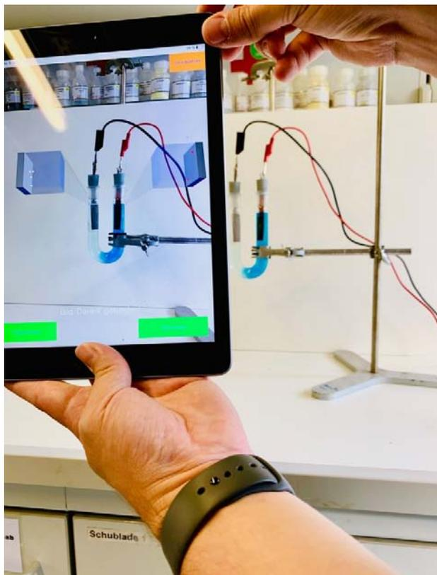
**Figure 14.** Augmented Reality of the microscopic level in a Daniell element
