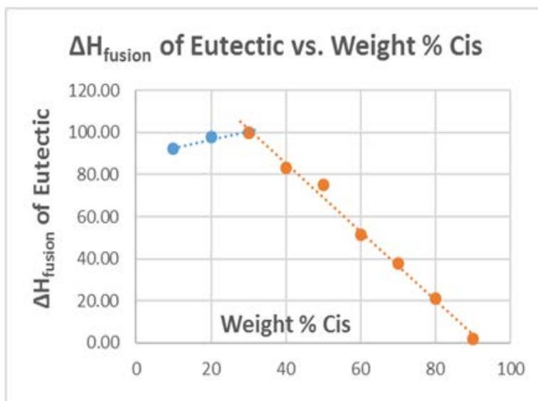
**Figure 5.** A plot of the eutectic peak enthalpy of fusion ( $\Delta H$ ) versus wt % cis isomer composition. The maximum corresponds to the eutectic composition (30 wt % cis isomer) having the maximum enthalpy of fusion of 100.1 J/g
