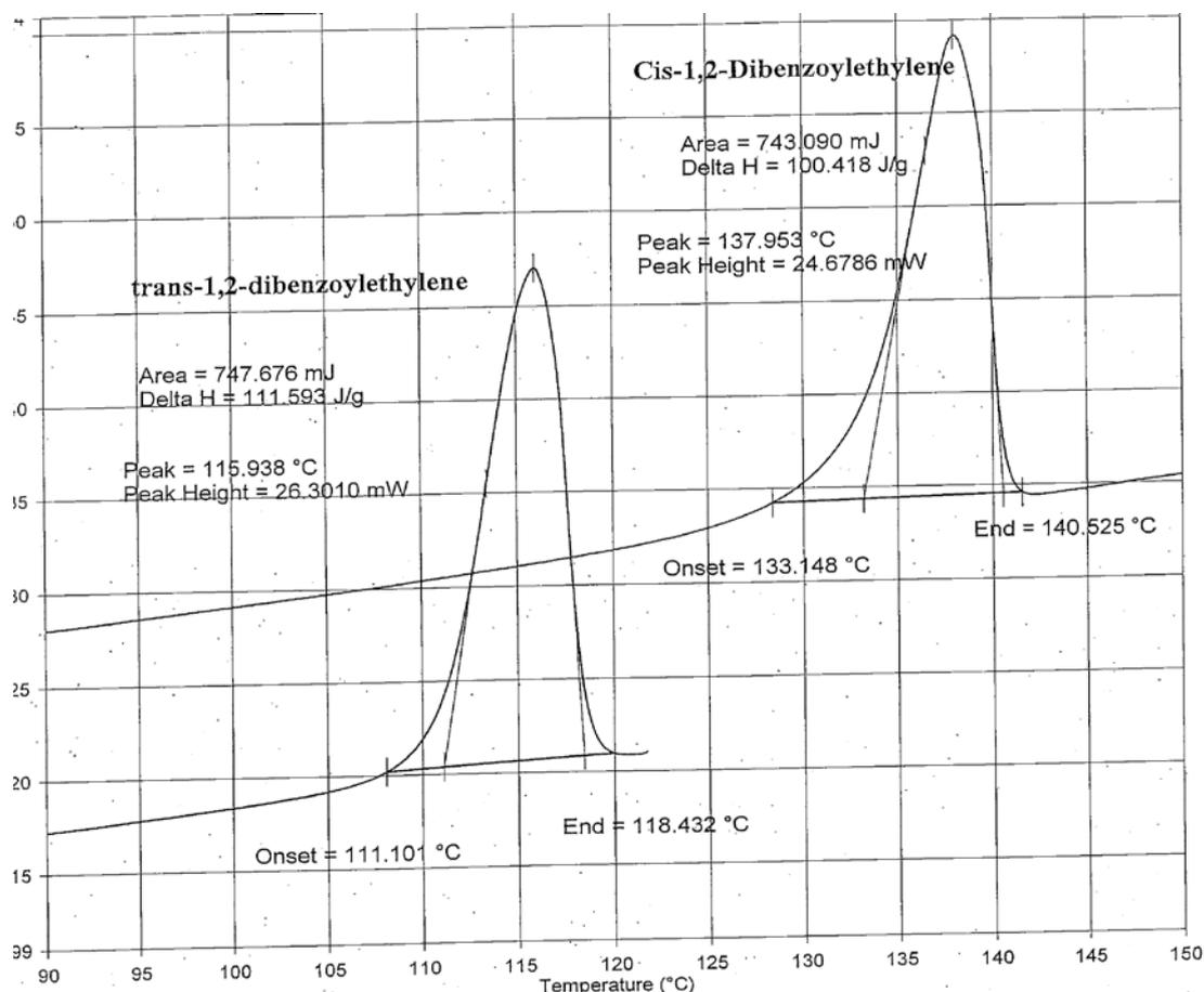
**Figure 2.** DSC thermogram of pure trans and cis isomer of 1,2-dibenzoyl ethylene showing the onset, peak, and end temperatures of melting and enthalpy of fusion
