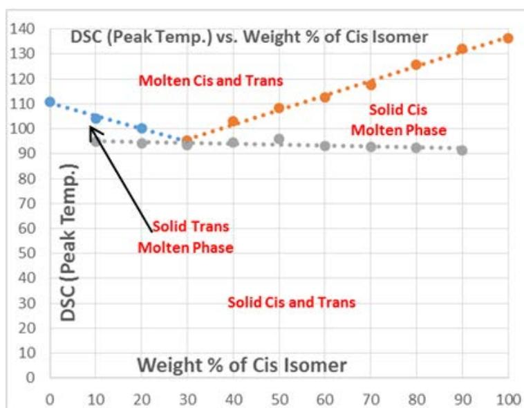
**Figure 4.** Phase diagram for the binary system of cis and trans isomer of 1,2 dibenzoyl ethylene. The binary phase diagram shows both the liquidus and solidus lines. The point of intersection of the cis liquidus and the trans liquidus line corresponds to the eutectic composition
