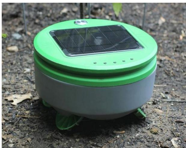
**Figure 4.** Solar lawn weeder for slashing weeds in lawn [4]
