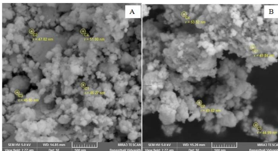
Figure 6. SEM image of Ni-doped CdS with doping concentration 2% (A) and 4% (B)
