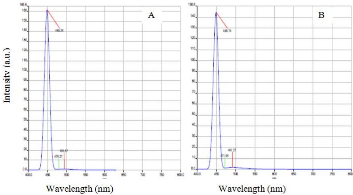
Figure 4. Photoluminescence (PL) spectra of Ni-doped CdS with doping concentration 2% (A) and 4% (B)
