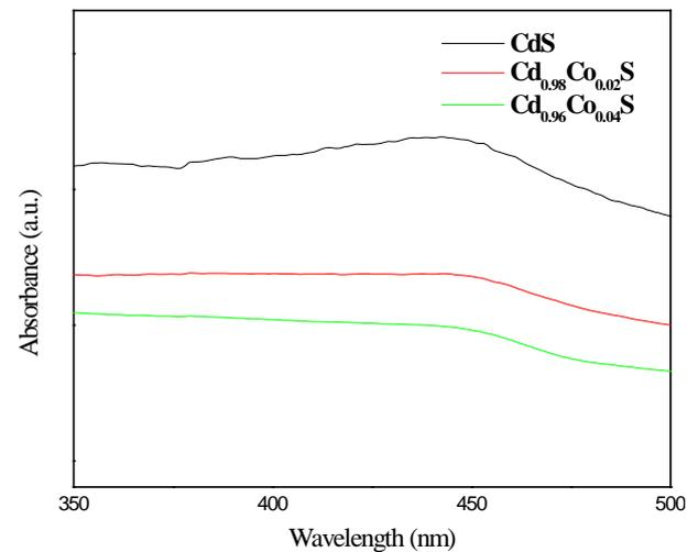
Figure 1. Absorption spectra for  $\text{Cd}_{1-x}\text{Co}_x\text{S}$  ( $x = 0, 0.02$  and  $0.04$ )
