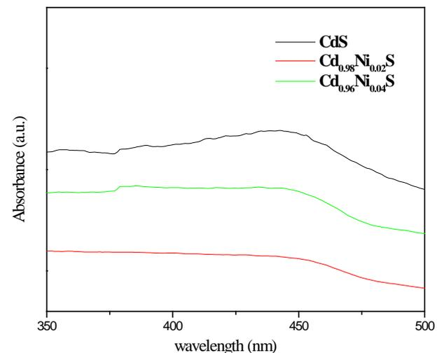
Figure 2. Absorption spectra for  $\text{Cd}_{1-x}\text{Ni}_x\text{S}$  ( $x = 0, 0.02$  and  $0.04$ )
