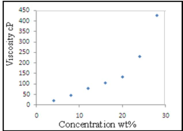
Figure 2. Solution viscosity as a function of nylon 6/ formic acid solution concentration
