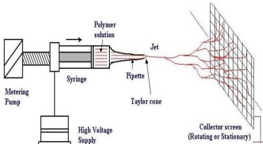
Figure 1. Line diagram of electro spinning assembly
