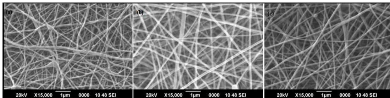
Figure 3. SEM images of electrospun nylon fibre (a) 16wt% concentration, (b) 20 wt% concentration and (c) 24wt% concentration.
