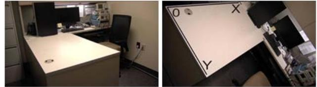
**Figure 6.** Left- and right-view images of the testbed. World coordinate system is defined on the testbed (overlaid for visualization on the right-view image.)
