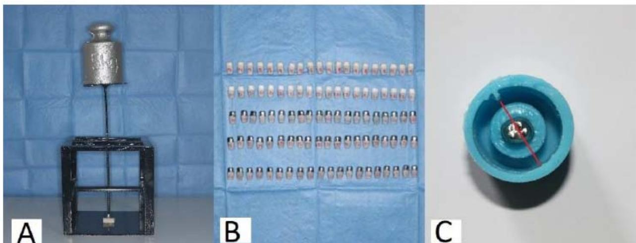
Figure 1. A = Cementation with 50N force, B = Cemented Specimens, C = Silicon pattern and cutting line
