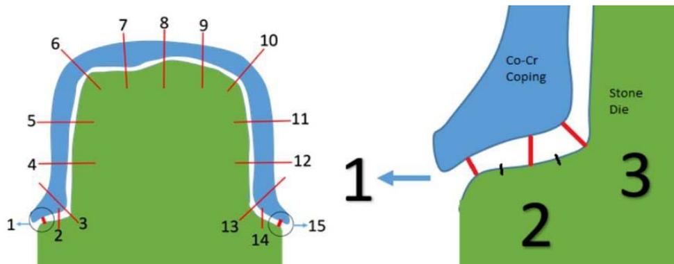
Figure 4. Marginal Gap (MG)(1. and 15. points), Chamfer step gap (CSG)( midpoint of step) ( 2. and 14. points), Chamfer Angle Gap (angle bisector) (CAG) (3. and 13. points), Axial Wall Gap (AWG) (4.,5.,11. and 12. points), Axio-occlusal Angle Gap (AOG), Occlusal Gap (OG) (7.,8. and 9. points)
