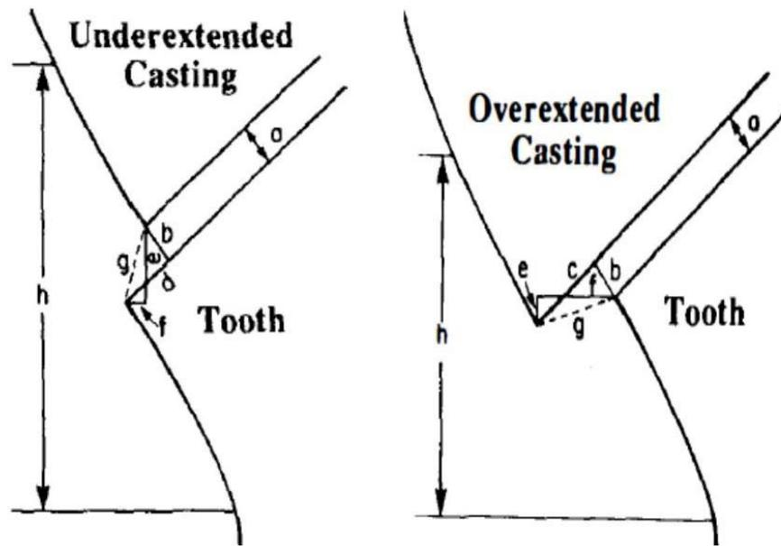
Figure 3. Casting misfit terminology. a = internal gap, b = marginal gap (measured in the this study), c = overextended margin, d = underextended margin, e = vertical marginal discrepancy, f = horizontal marginal discrepancy, g = absolute marginal discrepancy, h = seating discrepancy
