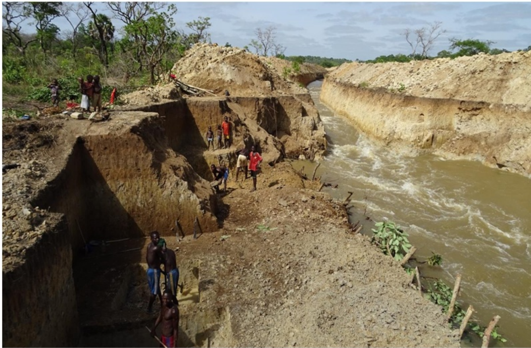
Photo 1. Opportunistic artisanal exploitation on the banks of the canal dug by Chinese mining companies to divert the Ouham River and exploit its dry bed, near Bozoum
