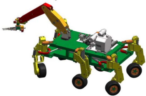
Figure 3. 3D model of the complex modular robotic system [4]
