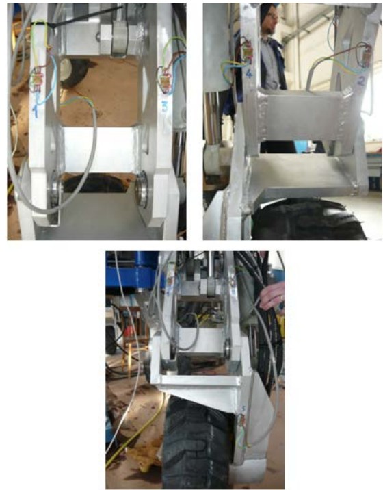
Figure 10. Applied strain-gages in places 1 to 5
