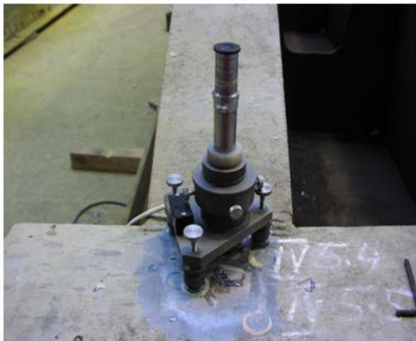
**Figure 12.** Measurement of residual stresses by system RS 200
