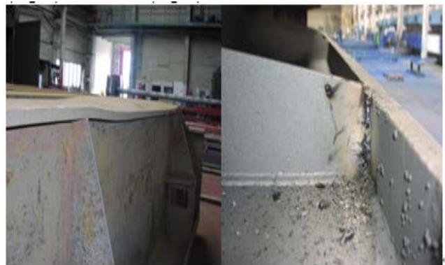
Figure 5. Deformation of flange and poor weld
