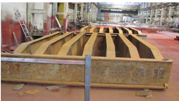
Figure 4. View to sluice gates
