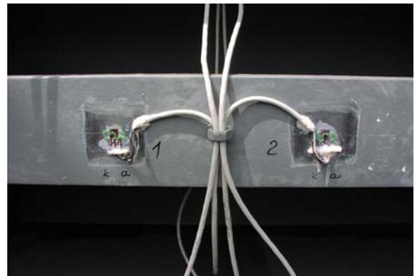
**Figure 14.** Detail of applied strain-gages
