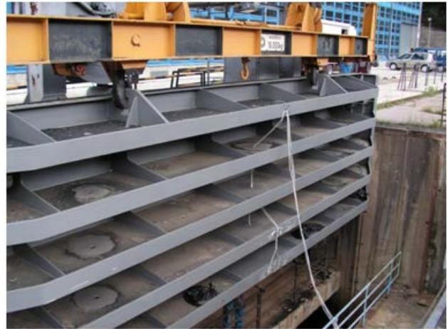
**Figure 13.** Insulated strain gages on sluice gate before measurement
