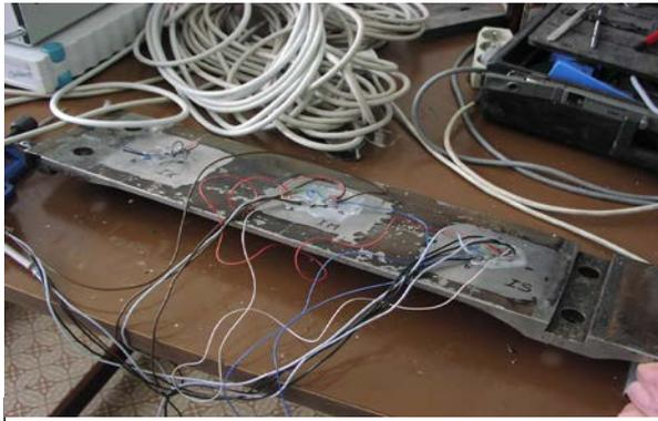
Figure 2. Locations of strain gages RY 61 for the hole-drilling method measurement
