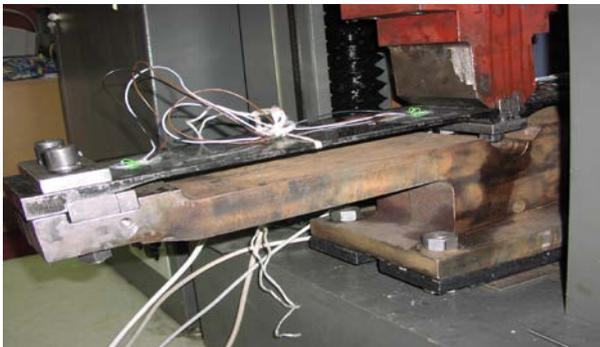
Figure 4. Leaf spring with applied strain gages in tensile test machine
