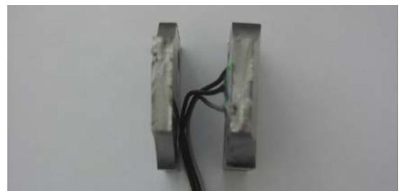
Figure 13. Fracture surface of specimen 1
