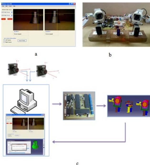
Figure 8. a) C# 3D scanner program, b) RRP 3D scanner and c) 3D scan of surface algorithm
