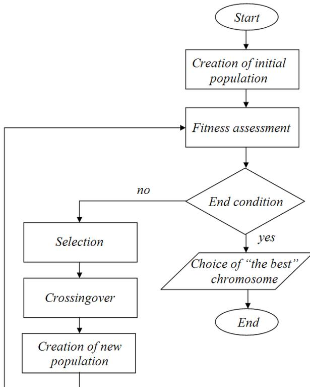
Figure 1. The flowchart of genetic algorithm of finding of an optimum technological route
