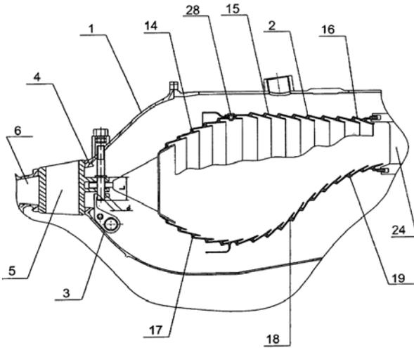
**Figure 10.** General view of a diffuser of the combustion chamber of the aviation engine (the position 5 - detail 'Rack')
