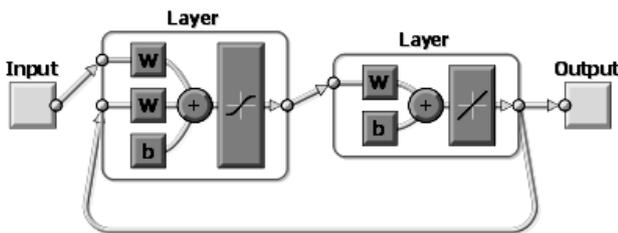
Figure 4. The Jordan's networks scheme for the solution of a problem of multicriteria optimization of resources savings perspective technological processes in the environment of MATLAB
