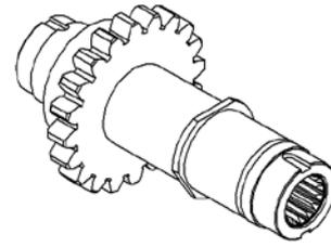
Figure 5. 3D model of detail-representative "gear wheel"
