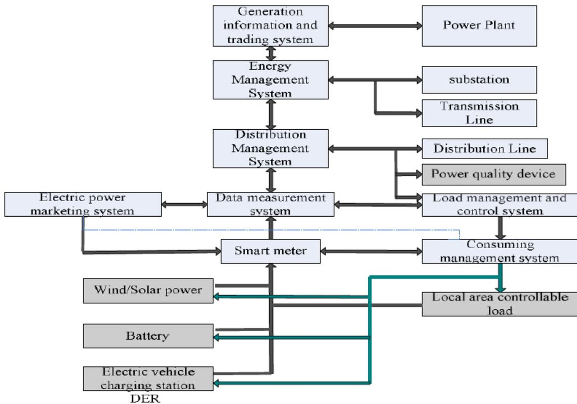
Figure 4. Detailed Information flow of DSM with other management units
