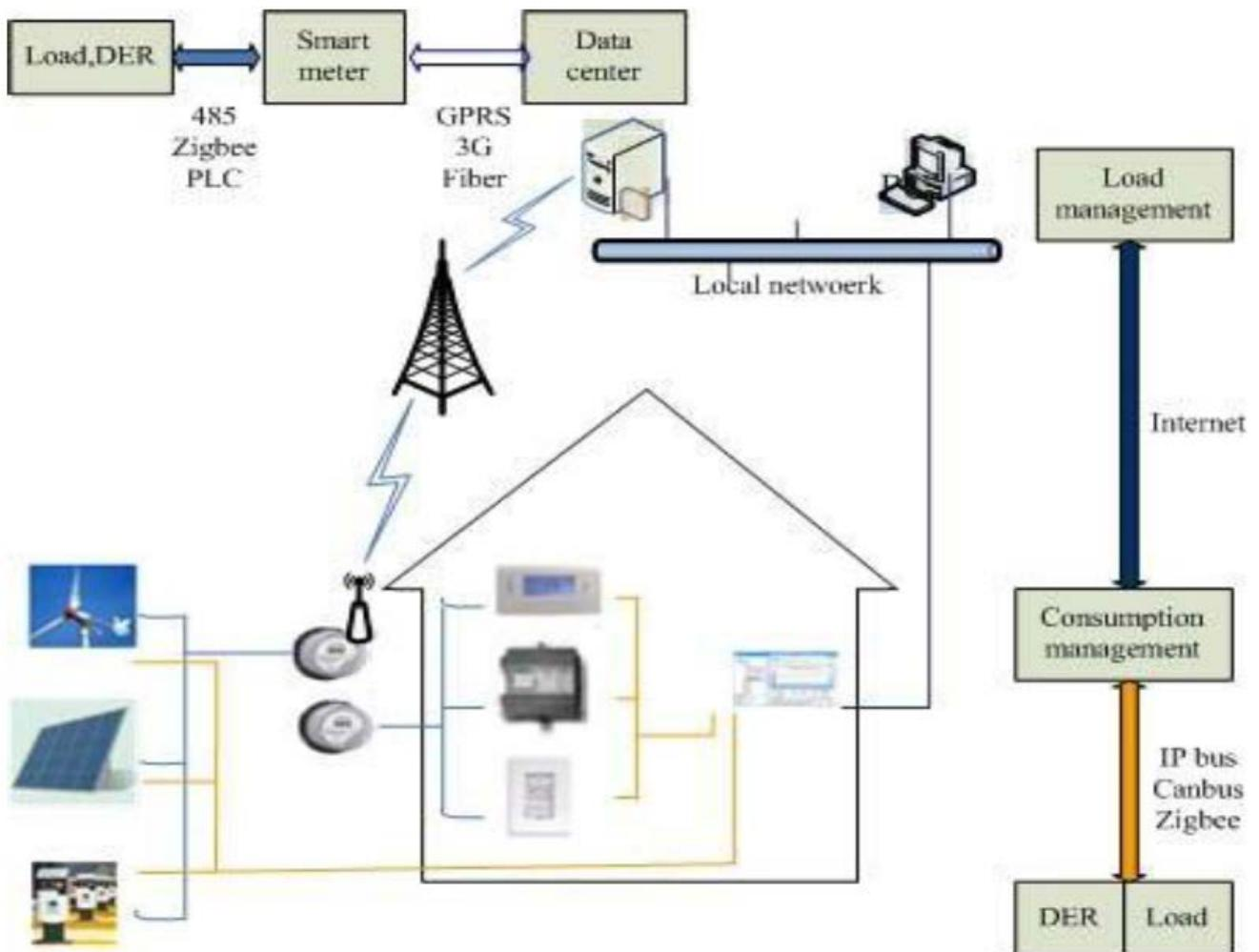
Figure 5. The communication grid in DSM framework
