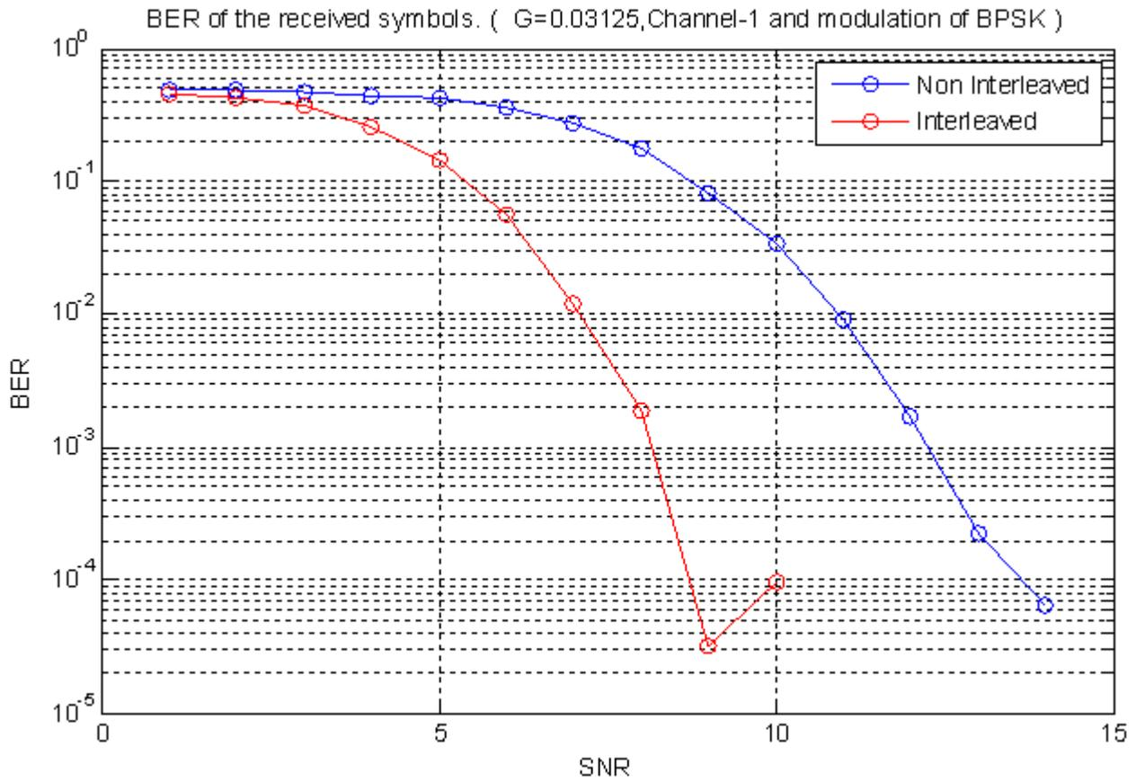
Figure 6. Effect of Block interleaver in BPSK on Channel-1
