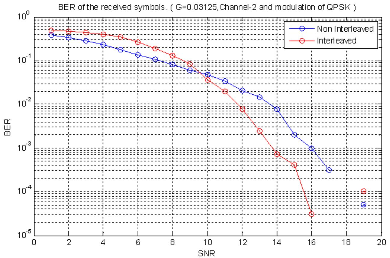
Figure 9. Effect of Block interleaver in QPSK on Channel-2
