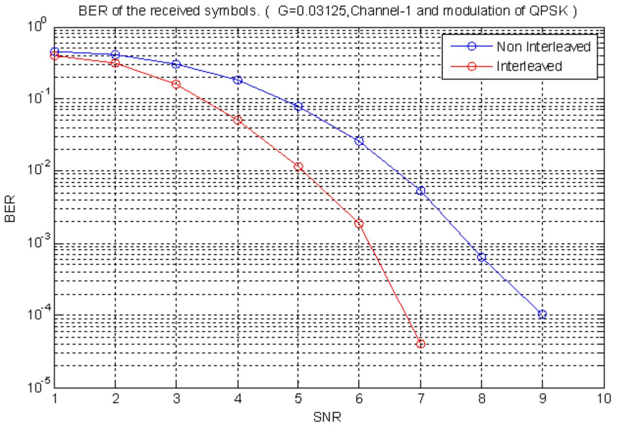
Figure 8. Effect of Block interleaver in QPSK on Channel-1
