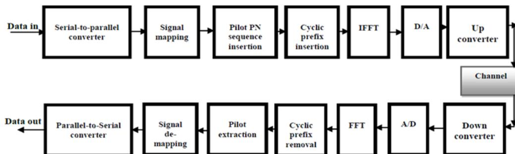
**Figure 1.** Block diagram of an OFDM Transceiver
