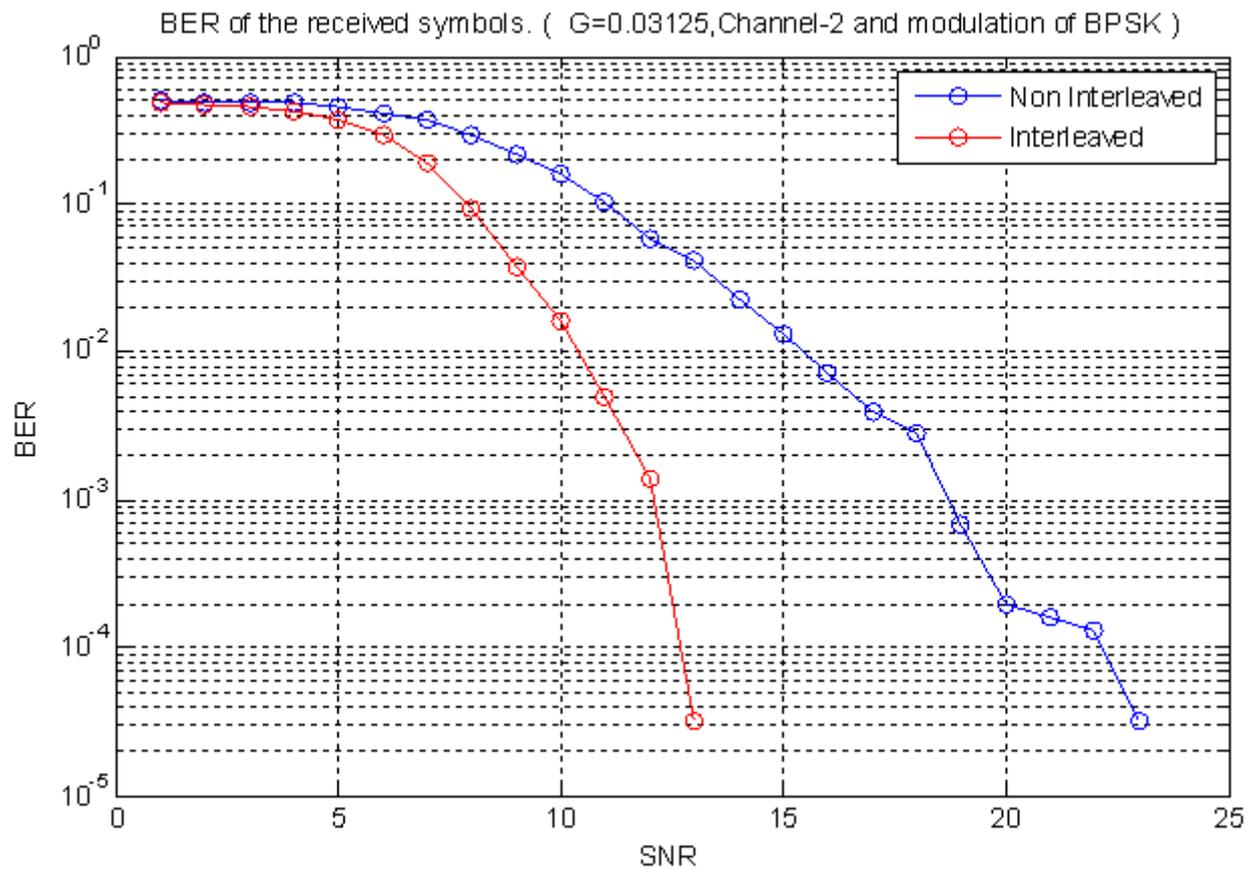
Figure 7. Effect of Block interleaver in BPSK on Channel-2
