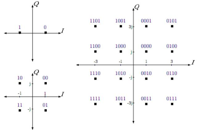
Figure 5. BPSK, 4-QAM, and 16-QAM constellation diagrams [10]
