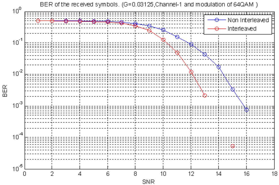
Figure 12. Effect of Block interleaver in 64-QAM on Channel-1
