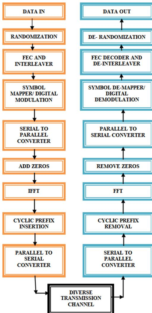
Figure 2. Simulation model of WiMAX-PHY layer
