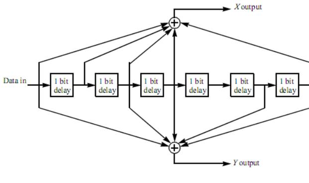
Figure 4. Convolutional Encoder of mother code rate  $\frac{1}{2}$  [3]
