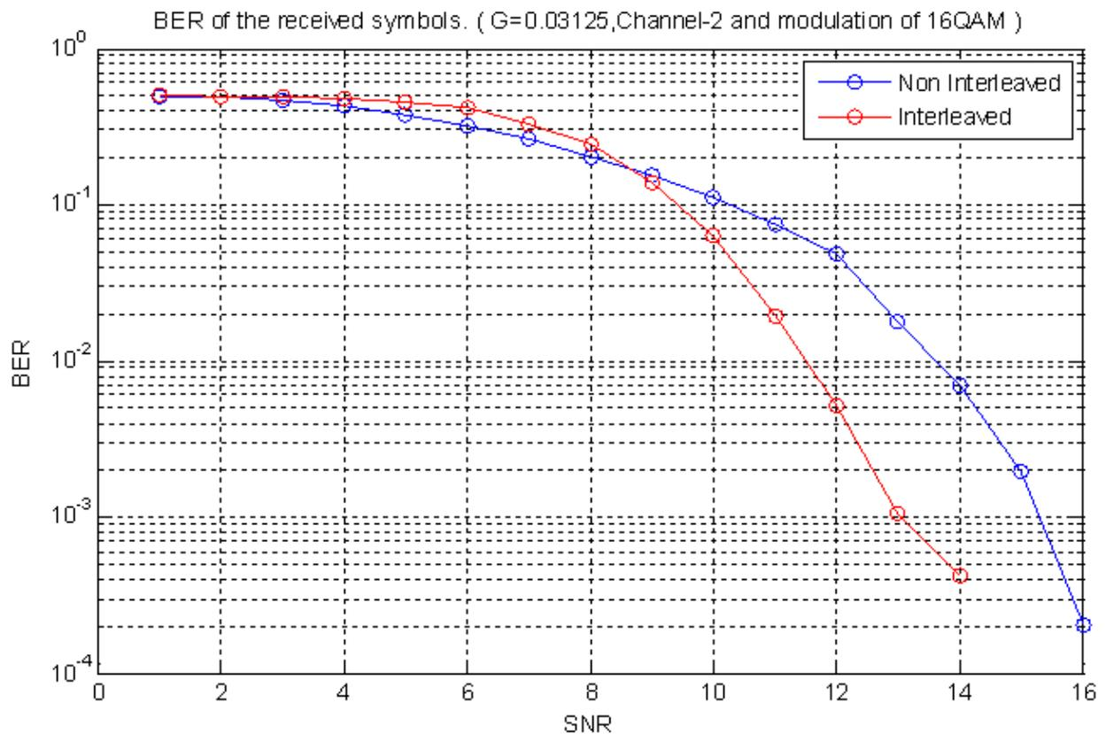
Figure 11. Effect of Block interleaver in 16-QAM on Channel-2
