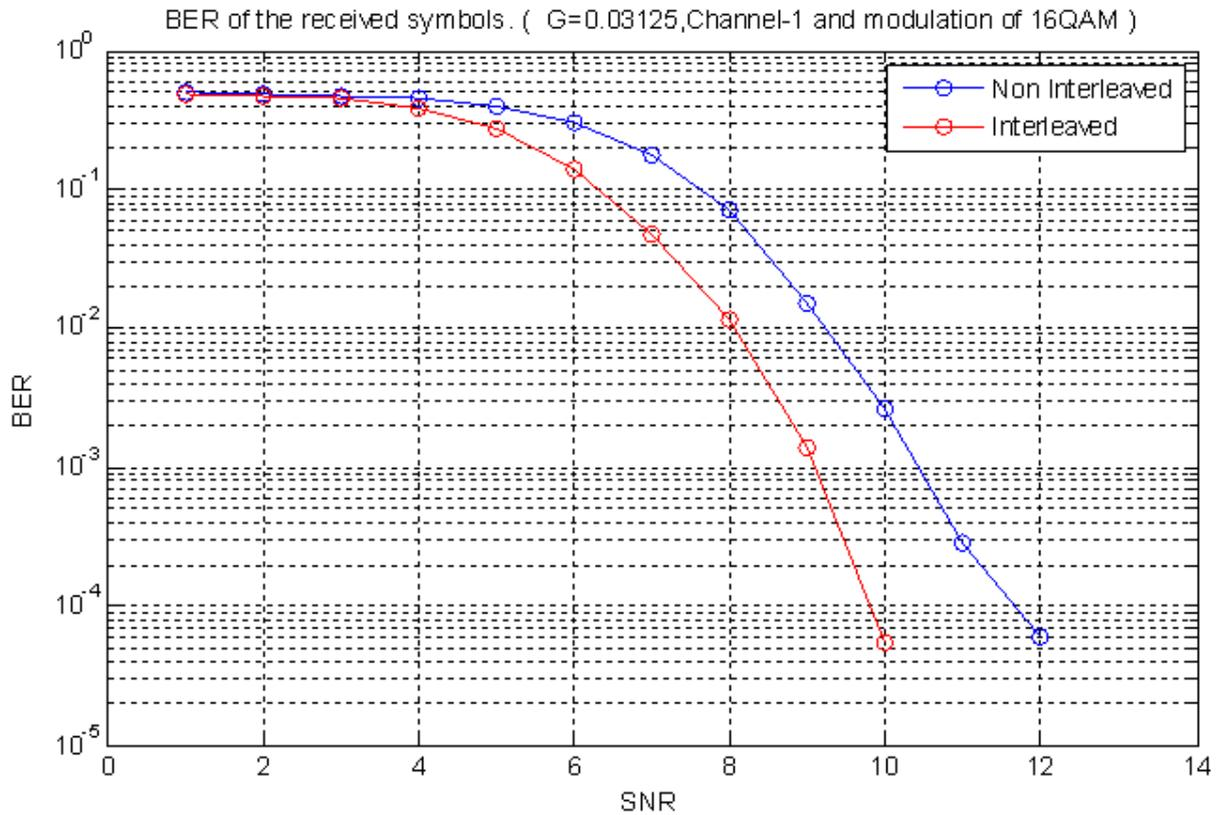
Figure 10. Effect of Block interleaver in 16-QAM on Channel-1
