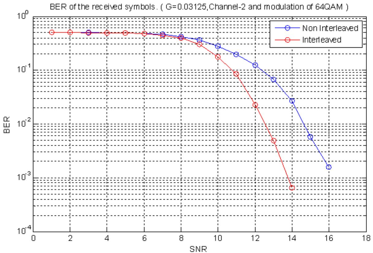
Figure 13. Effect of Block interleaver in 64-QAM on Channel-2
