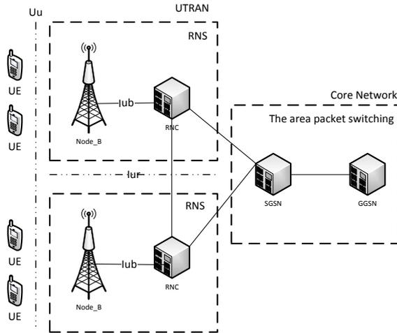
Figure 1. Architecture of the UMTS network
