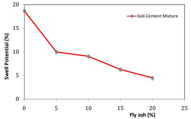
Figure 5. Effect of Cement-Fly ash on Swell Potential
