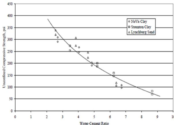
Figure 2. Relationship between 28-day Unconfined Compression Strength and Water-Cement Ratio (source [16])
