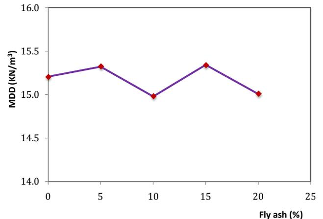
Figure 7. Effect of Cement-Fly ash on Maximum Dry Density (MDD)
