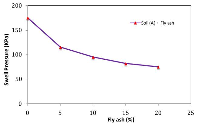
Figure 6. Effect of cement-Fly ash on Swell Pressure
