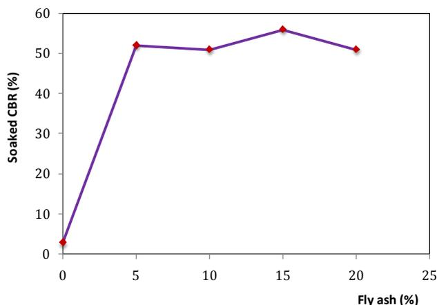
Figure 9. Effect of cement-fly ash on soaked CBR
