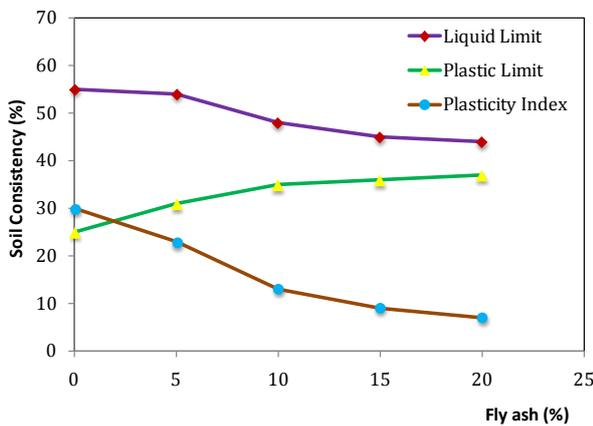
Figure 4. Effect of cement-fly ash on soil consistency
