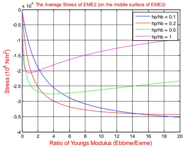
Figure 17(b). Average stress of the EME2 layer (on the middle surface of the EME2)
