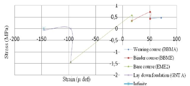
Figure 13. Variation of shear stresses function of the deformations
