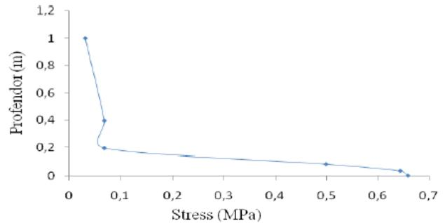
Figure 11. The dissipation of the normal stress for the various layers
