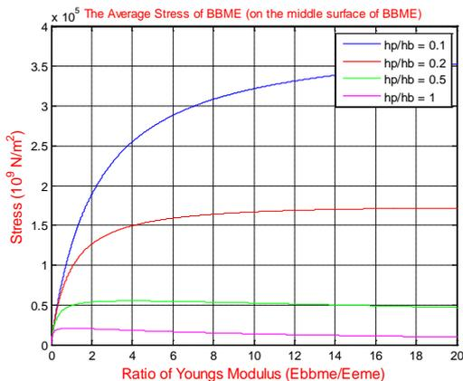
Figure17 (a). Average stress of the BBME layer (on the middle surface of the BBME)
