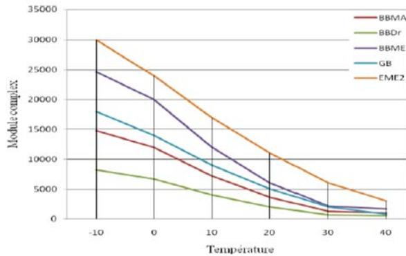
Figure 9. Influence of the temperature on the modulus complex
