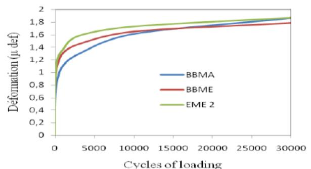
Figure 5. Deformation with rutting according loading
