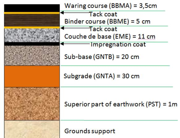
**Figure 1.** Roadways with multi-layer structure used for the EAST-WEST highway
