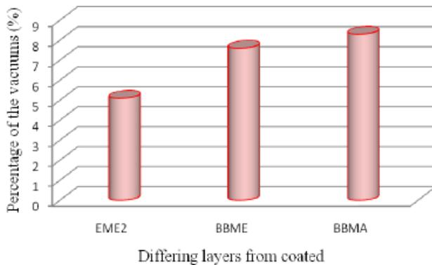
Figure 7. Percentage of the vacuum for differing layers from coated
