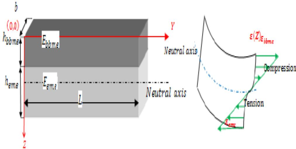
Figure 2. Section and normal distribution of constraint
