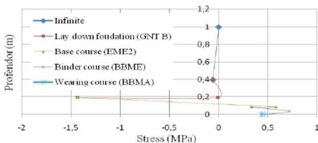
Figure 10. The dissipation of shear stresses for the various layers
