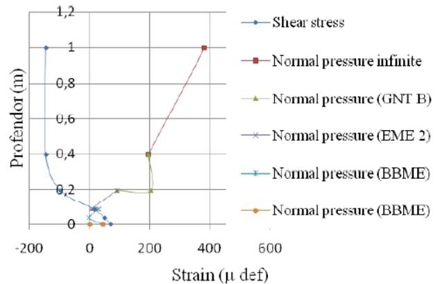
Figure 12. Distribution of the normal deformations and sheerings
