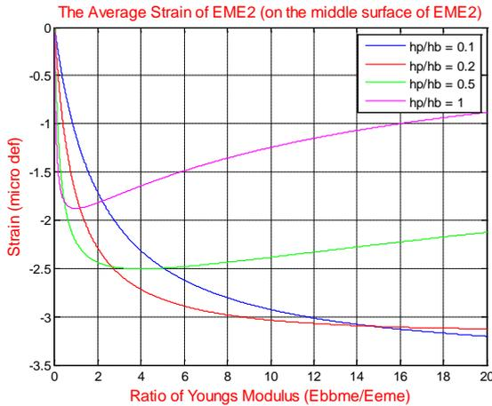
Figure 15. Average strain of the EME2 layer (on the middle surface of the EME2)
