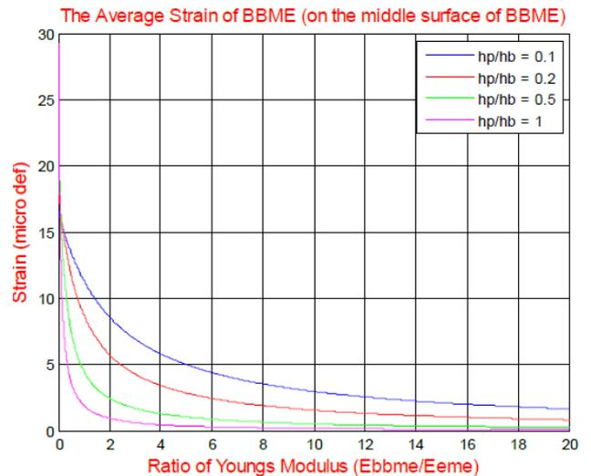
**Figure 14.** Average strain of the BBME layer (on the middle surface of the BBME)
