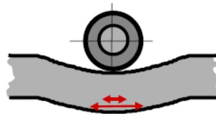
Figure 16. Cracking in inflection with the interface of the two layers
