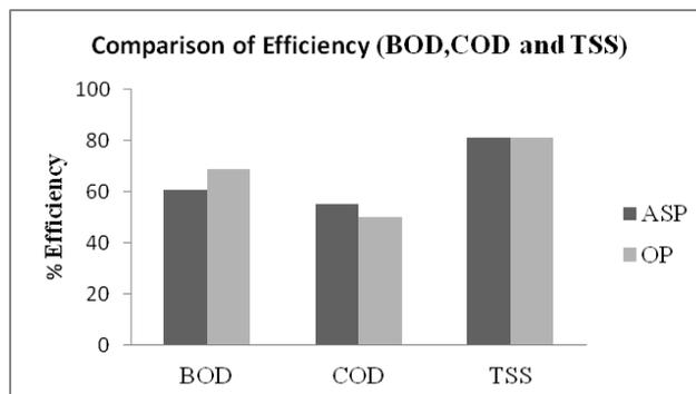
**Figure 1.** Efficiency of ASP and OP for BOD, COD and TSS removal
