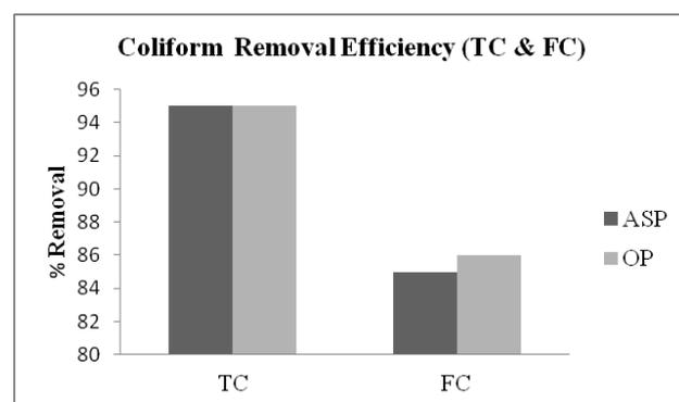
**Figure 2.** Total and Fecal coliform removal efficiency of ASP and OP
